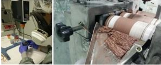
Figure 1: Ink being mixed in the overhead stirrer (left) and homogenized at the three roll mill (right).
