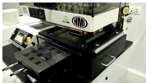
**Figure 3.** Screen printing process for a contact metallization.
