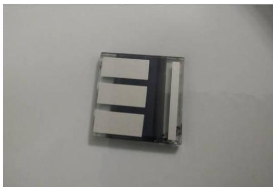
**Figure 5.** Sample of perovskite solar cell.
