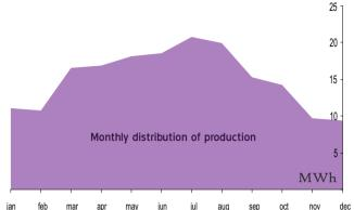
Installed power 100 kW Generated Energy in the year 181 Mwh ITER participation 100 % Equivalent consumption 214 persons Tons of CO<sub>2</sub> emissions avoided 101 tons
