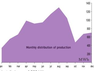
Installed power 4.800 kW Generated Energy 9.750 Mwh ITER participation 50 % Equivalent consumption 11.541 persons Tons of CO $_{\!\scriptscriptstyle 2}$  emissions avoided 5.414 tons
