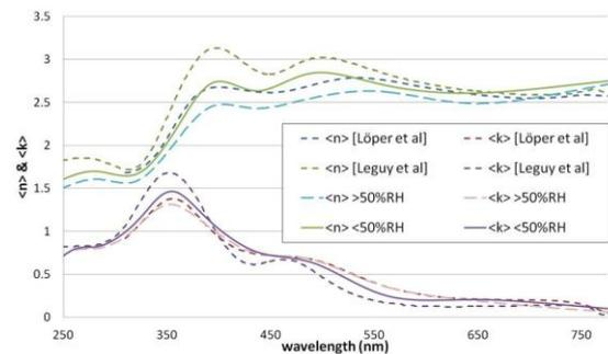
**Figure 2:** Comparison of the refractive index and the extinction coefficients.
