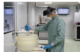
Figure 4: Spin coating process for the layers deposition
