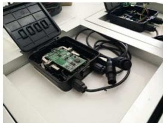
Figure 3: View of a mini-module with the junction box opened showing the acquisition card assembled
