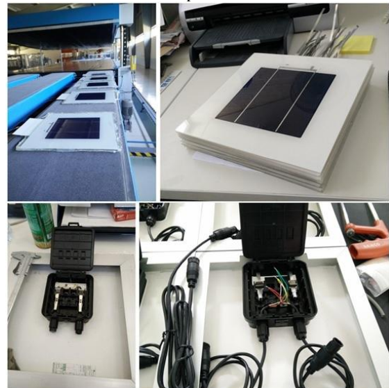
Figure 1: View of the one-cell modules after lamination (up-left), trimming operation (with exposed circuit terminals, up-right), frame (down-left) and junction box attachment (down-right).
