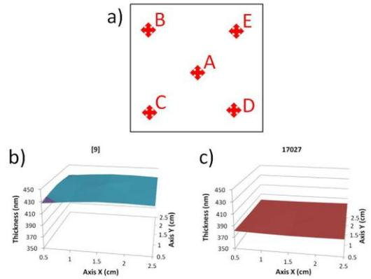
**Figure 5:** Measurement points (a), perovskite thickness distribution of samples from previously published results (b) and fabricated by current methodology (c).
