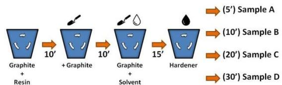
**Figure 3:** Mixing procedure.
