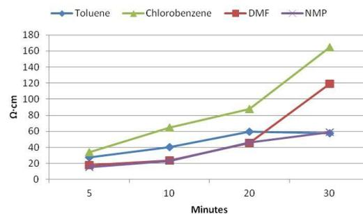
**Figure 8:** Resistivity measured in the contacts deposited via Doctor blade.
