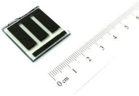
**Figure 1:** Example of a screen printed contact.
