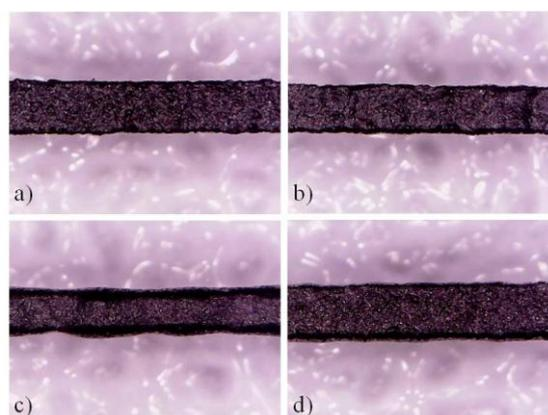
**Figure 9:** Microscope images showing contacts deposited by doctor blade with Toluene (a), Chlorobenzene (b), DMF (c) and NMP (d). All the contacts were deposited 20 minutes after adding the hardener
