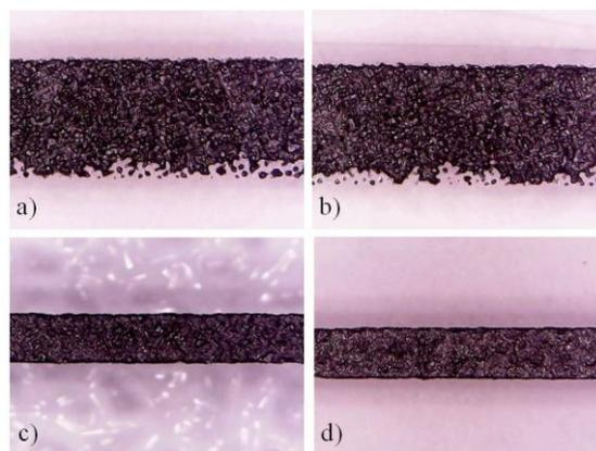
**Figure 11:** Microscope images showing contacts deposited by screen printing with DMF (a) and NMP (b) as well as doctor blade with DMF (c) and NMP (d). All the contacts were deposited 20 minutes after adding the hardener
