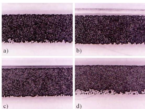
**Figure 7:** Microscope images showing contacts deposited by screen printing with Toluene (a), Chlorobenzene (b), DMF (c) and NMP (d). All the contacts were deposited 20 minutes after adding the hardener.
