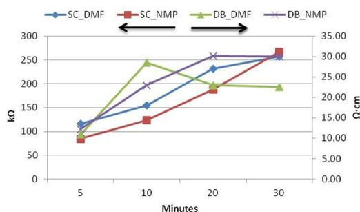
**Figure 10:** Resistance and resistivity measured in the contacts deposited via screen printing and doctor blade, respectively.
