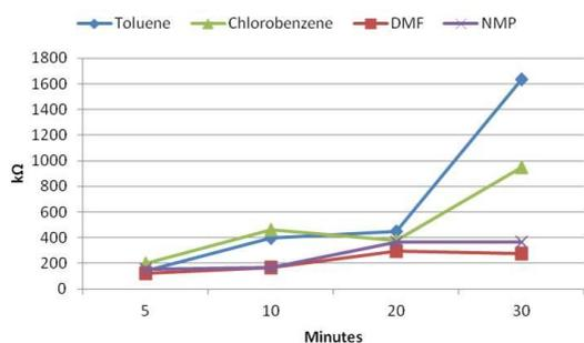
**Figure 6:** Resistance measured in the contacts deposited via screen printing.
