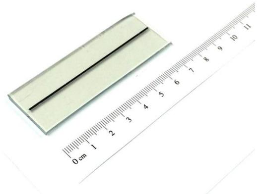
**Figure 2:** Example of a doctor blade printed contact.
