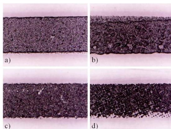
**Figure 4:** Microscope images showing contacts deposited by screen printing with inks M19 (a), M21 (b), M22 (c) and M23 (d).
