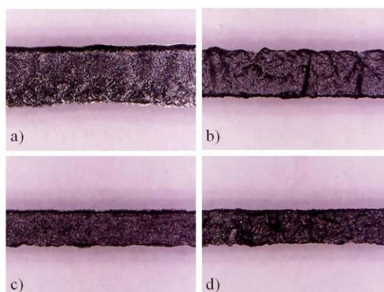
**Figure 5:** Microscope images showing contacts deposited by doctor blade with inks M19 (a), M21 (b), M22 (c) and M23 (d).
